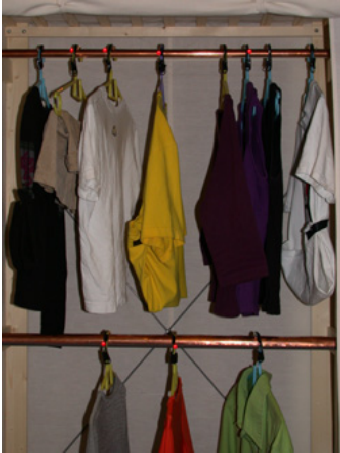
Figure 3: Wardrobe used in evaluation containing two Hanger Displays: top rod shows predicted high temperature (4 of 8 hangers are on, which indicates 15° C); bottom rod alternates between showing remote presence and barometric pressure (2 of 3 hangers are on, which, for the barometric pressure application, indicates a 75% chance of rain).
